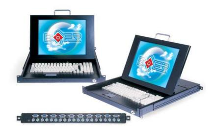
Controlling multiple PCs from one keyboard, mouse and VGA monitor, the KVM-9000 is loaded with such features as 19" rackmount size, daisy chain up to eight units, On Screen Display menu, password security, PC server name search, hot key control, front panel push button and auto scan control. It has a complete keyboard and mouse emulation for simultaneous PC boot-up process.
